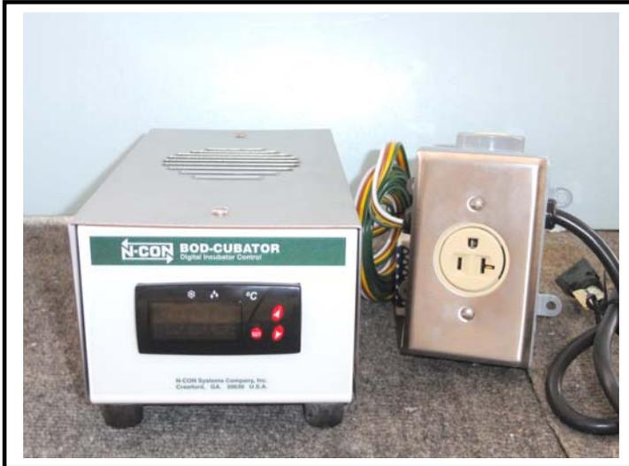
The N-CON BOD-Cubator Incubator Control converts any new or used refrigerator, from under-counter to the largest household size into a precisely controlled BOD incubator. No permanent modifications are necessary.\* You can temporarily convert a refrigerator to meet peak loads and then return it to normal use. By obtaining a refrigerator sized to meet your needs locally you can avoid high shipping costs and servicing headaches.
