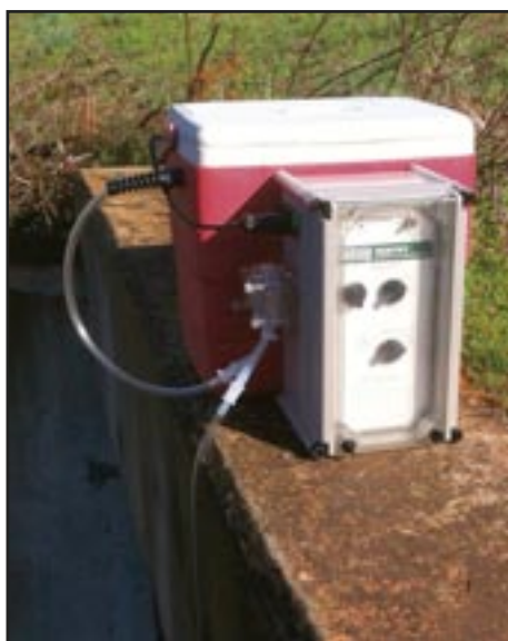
Operating in the field on a 12V battery mounted on a modified ice chest.
